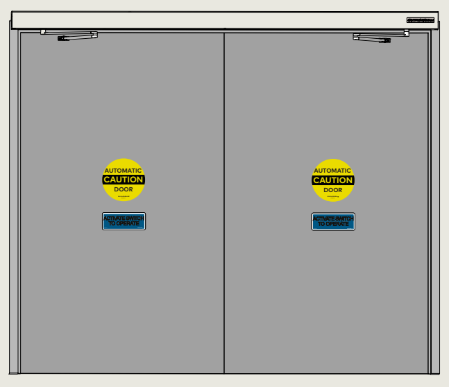
Fig. 6.8.3 Push/Pull, push to operate
